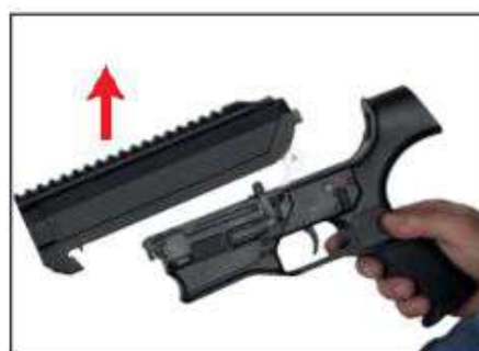
17. Remove the upper receiver but moving it forward.
