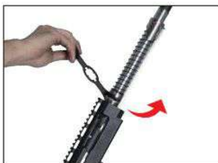
9. Use the wrench to unscrew the barrel nut. Rotate in clockwise direction.
