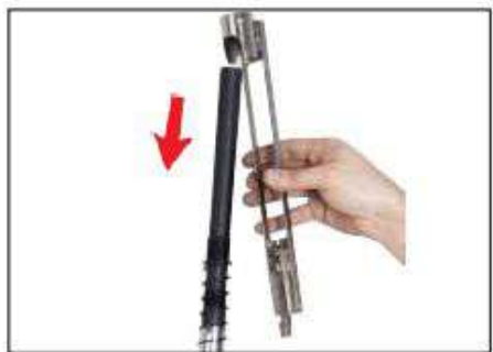
5. Insert the slide into the barrel so that the tube part of the slide stays up.
