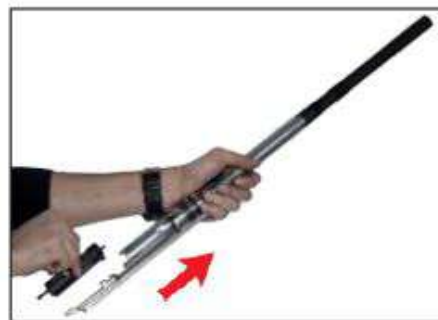
6. Pull the slide back by holding it firmly against the force of the spring and put the bolt on slide.
