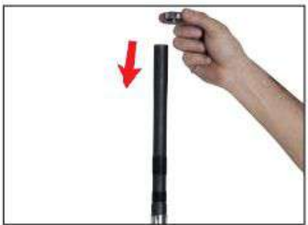
3. Barrel locking nut insert it into the barrel with the key slots facing up.
