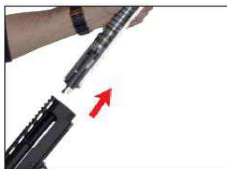
10. Unscrew the barrel nuts from the body. Make sure you take it apart. Barrel and slide holding it together and pulling it upwards from the body remove it.
