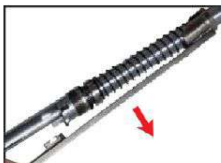
12. Pulling back the slide on the barrel take the bolt, free the slide from barrel and remove in the upward direction.
