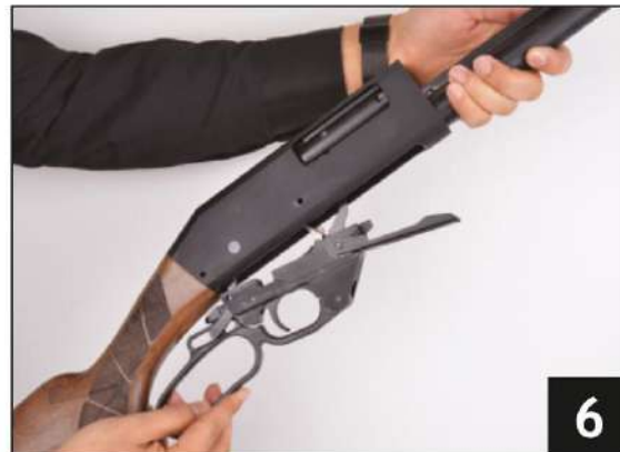
6 - Take out the trigger assembly by pushing it outside.
