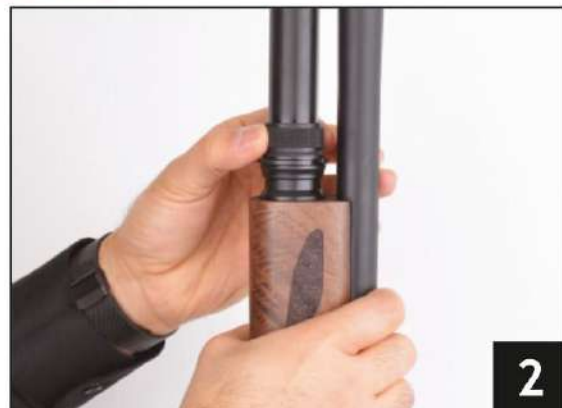
2 - Remove the forend cap by turn it to anti-clockwise.
