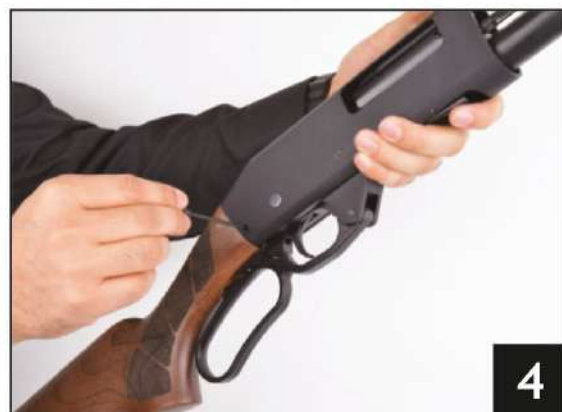
4 - Take down the receiver pins by pressing with external screw.
