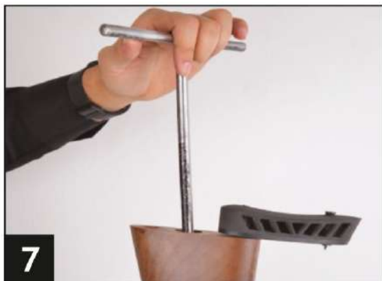
7 - First remove the screw of rubber pad and than take out the screw of stock/butt.
